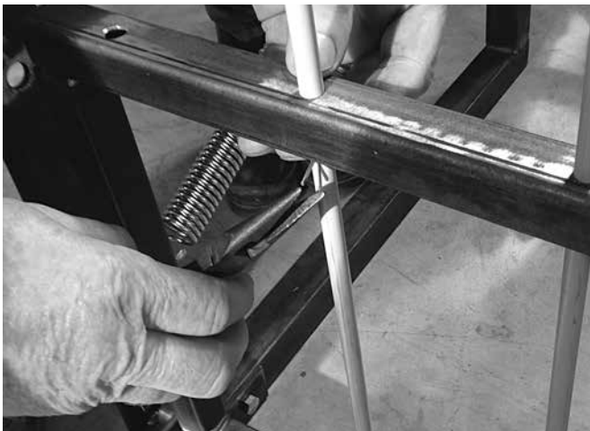
STEP 9. Secure each rod with a cotter pin through the small hole found in each rod just underneath the top bar of the SWING FRAME.
