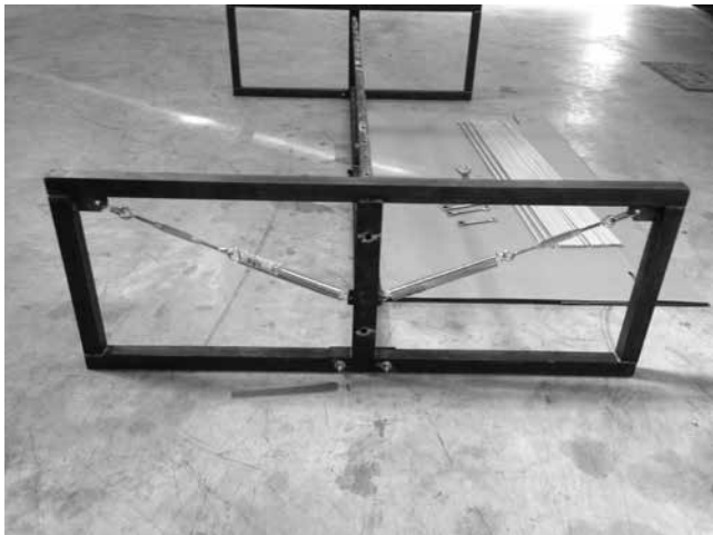
STEP 7b. The assembled SPRINGS and TURNBUCKLES
