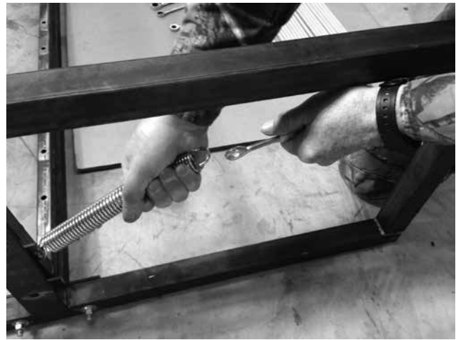
STEP 7a. Connect each SPRING to its TURNBUCKLE. Be sure to lessen the tension of the TURNBUCKLE to enable this step. NOTE: Once the gate is installed within your fence, use the turnbuckles to adjust the swing frame to a vertical position. This enables the gate to be used on unlevel ground.
